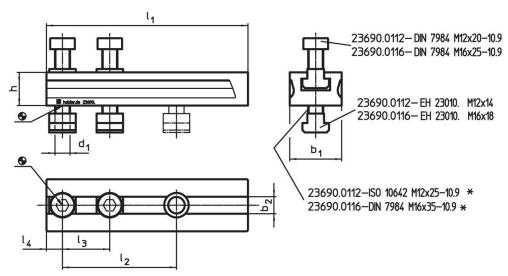
\* When using more height adapters the screws ISO 10642 or DIN 7984 have to be replaced by screws extended by the dimension h.
