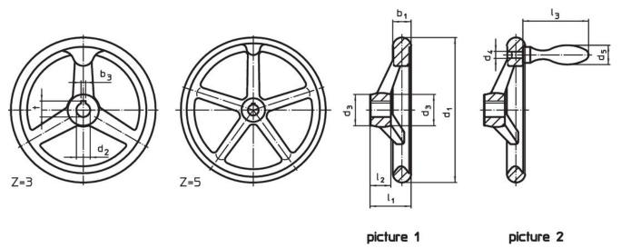
The orientation of the hub keyway may be different than shown in the drawing.
