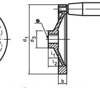
The orientation of the hub keyway may be different than shown in the drawing.
